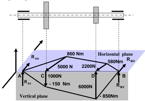
**Loading and Bending Moment Diagram**
